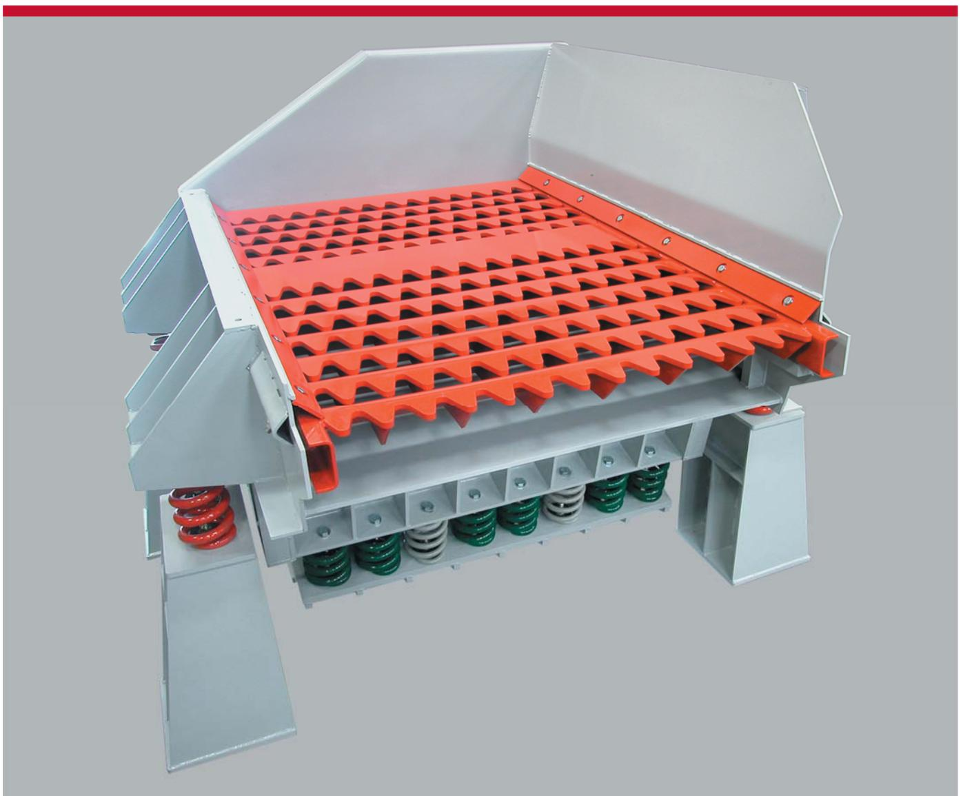
This Series 923 EZ-WERK™ Vibratory Shakeout by Dynamic Air is a natural frequency vibratory shakeout which handles up to 60 inch square by 30 inch high molds, weighing up to 10,000 pounds, at a rate of one every fifteen minutes. It uses the proven AR hardened finger deck for longer life. The molds are dumped from a mold dump onto the side of the shakeout to meet
