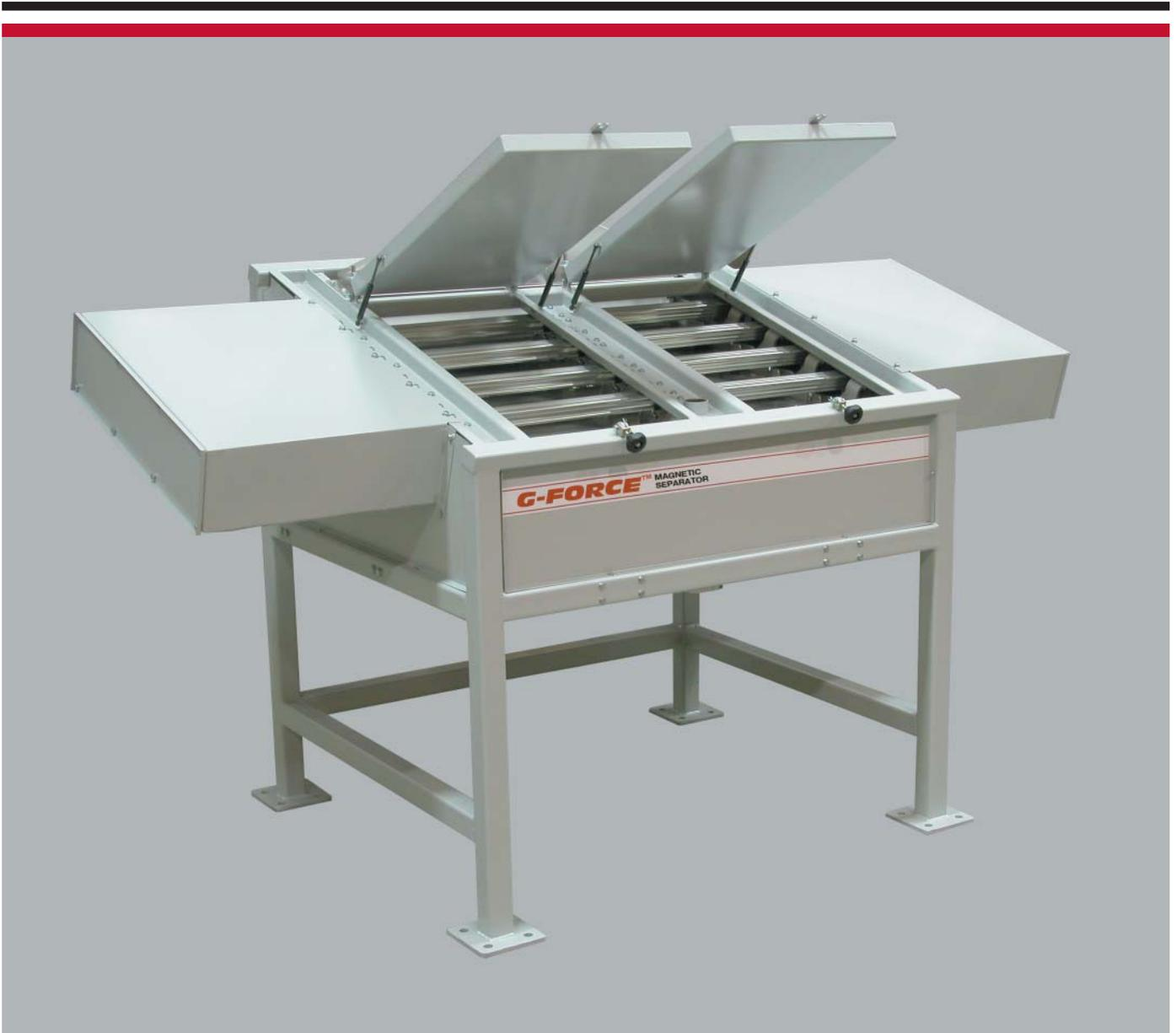
The G-Force™ Magnetic Separator by Dynamic Air was designed for magnetically separating fugitive metal particles from almost any dry bulk granular product, such as the removal of plastic pellets which may contain metallic particles. This particular model has the ability to operate continuously and contains multiple magnetic rods with automatic wipers to continually keep them clean of magnetic particles. The product flows through the separator using the
