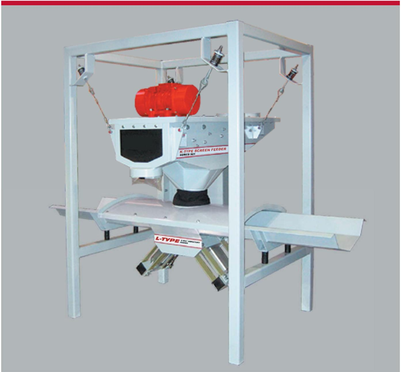
This Dynamic Air K-Type Vibratory Screen Feeder is used to convey material from a surge hopper into two different directions as required. The K-Type Screen Feeder screens sand down to 50 mesh
