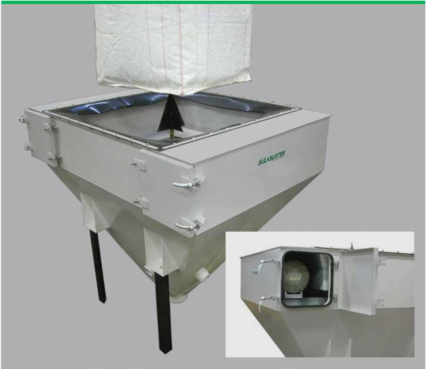
The Series 422 Model 2600 BulkBuster bulk bag unloader is designed to unload flat-bottomed bulk bags. It is a bulk bag unloader with discharge hopper and a fixed blade. It includes a dust collector with a support frame and can be loaded by a forklift or hoist. The weight of the bulk bag pierces the large bulk bag when it is lowered onto the fixed blade of the BulkBuster bulk bag unloader.
